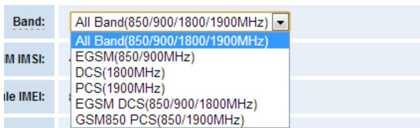
**Figure 3-1-3 Band Binding**
